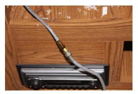
chance that if the metal barrel was to come in contact with the 120 voltage, it would conduct powr to the other electronics. Note the "tab" left on the end of the tape. This is for the future if
