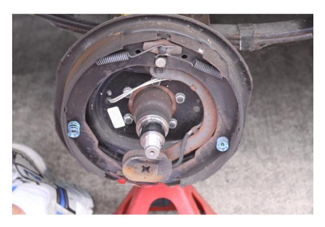
6. Install the new brake assembly on the studs sticking out of the axle and run the nuts down about hand tight. Using a torque wrench, tighten each nut (in a star pattern) to 50 foot pounds.
