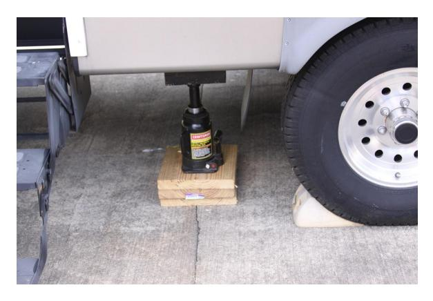
The picture above shows the jack, shoring, and the block between the jack and the frame of the trailer. The picture below shows the trailer on the jack stands with the wheels removed.
