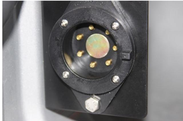
The other picture is the brass pins that make connect with the pins in the plug from the trailer. Stainless steel springs are used to keep the pins in connect. The projection on the side is an index mark required to line up the connection pin to pin relationship. Note that there isn't a center connection. All connections are around the circumference of the socket and plug.
