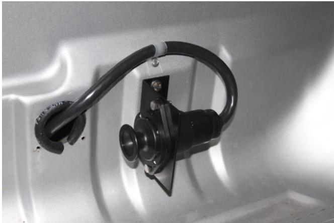
This is a picture of the installation in the bed of our 2005 Ford F-250. The plug section is mounted against the side wall of the bed for two reasons. First the plug was too deep to fit in the gap between the inner and the outer walls of the bed. The second is that I wanted the connection to come apart if I forgot to disconnect without damage.
