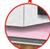
Air space left between tanks and bottom to protect against freezing
