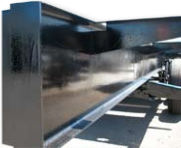
Welds along main rails create camber
