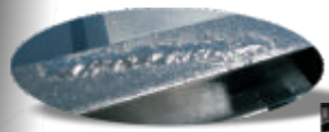
Additional Welds Create Camber in the Chassis for Greater Load Carrying Capacity
