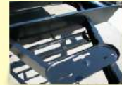
Welded LP /Battery Rack Sliding Battery Tray on 5th Wheels (most models)
