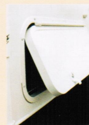
1" insulated and locking exterior storage compartments are finished with smooth fiberglass and sealed with an all-weather rubber gasket. Access is simplified with the handy finger pull and metal exterior door catch.
